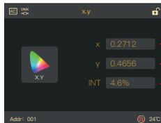
X-coordinate, switch the CCT/Hue knob to adjust from 0.2000 to 0.8000
