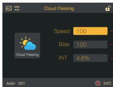
Speed, switch the CCT/Hue knob to adjust from 1 to 100
